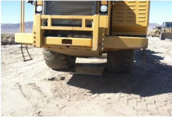
Photo 1: A drip pan is utilized beneath construction equipment.
