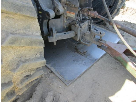
Photo 5: Drip-pans are being placed beneath equipment being stored overnight to ensure equipment does not leak directly onto the ground surface.
