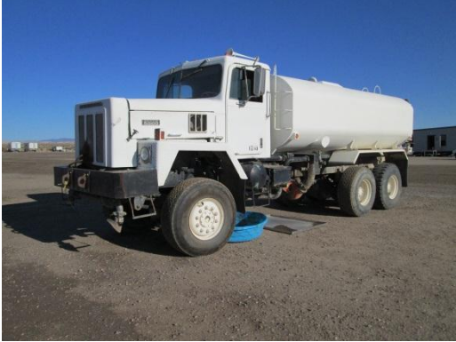
Photo 5: Crews place containment bins beneath construction equipment while not in use to prevent leaking equipment from leaking directly onto exposed soils.
