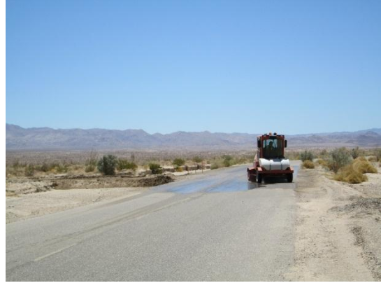
Photo 2: A mechanical sweeper is utilized to clean track-out along paved roadways that intersect with access roads for wind turbines.
