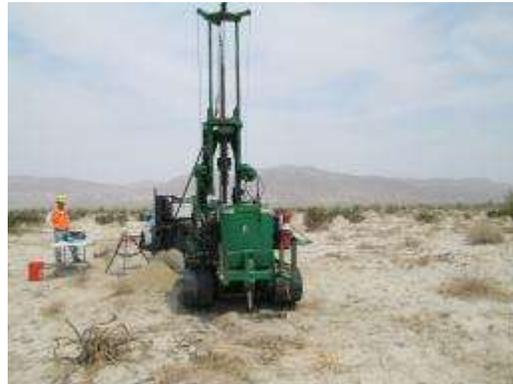
**Photo 8:** A crew completes geotechnical investigations at a wind turbine pad site in accordance with MM-Soils-1 and PHS-3.
