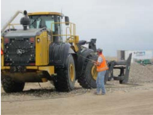
**Photo 5:** Construction crews wash wheel wells and tires on heavy construction equipment in accordance with the Integrated Weed Management Plan (MM-Veg-1d).
