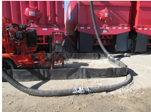
Photo 4: Secondary Containment is utilized on site for staged heavy equipment in accordance with best management practices identified in the SWPPP.
